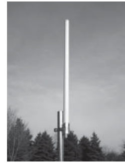
Multiple band MMO24580608 omnidirectional antenna
